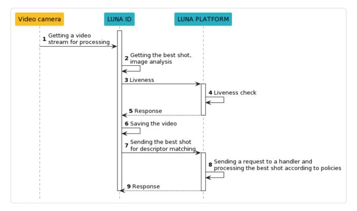
As the diagram shows, the process of interaction between LUNA ID and LUNA PLATFORM 5 is a back-and-forth communication between the frontend and backend.
