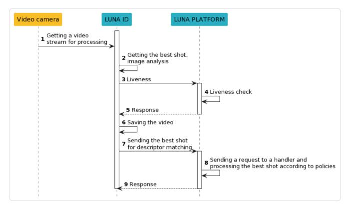
As the diagram shows, the process of interaction between LUNA ID and LUNA PLATFORM 5 is a back-and-forth communication between the frontend and backend.
